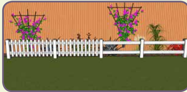
5. Fit rails or picket panels as desired (will slot into place).
